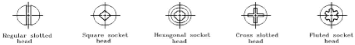
Figure 1-14 Different types of screw head slots
